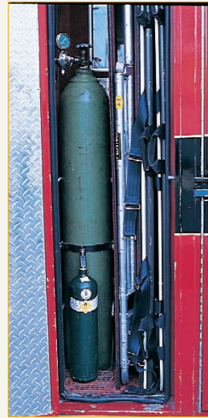
Figure 7-22 The cylinders that are most commonly found on an ambulance are the D (or super D) and M size cylinders.
