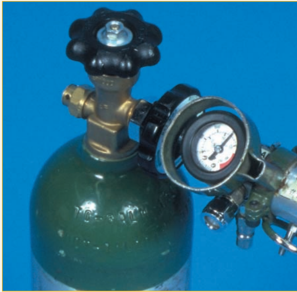
Figure 7-21 Oxygen tanks for medical use will have a series of letters and numbers stamped into the metal on the collar of the cylinder.
