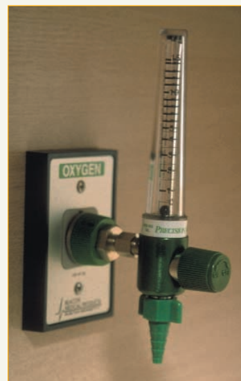
Figure 7-26 A pressure-compensated flowmeter contains a float ball that rises or falls according to the gas flow within the tube. It must be maintained in an upright position for an accurate reading.
