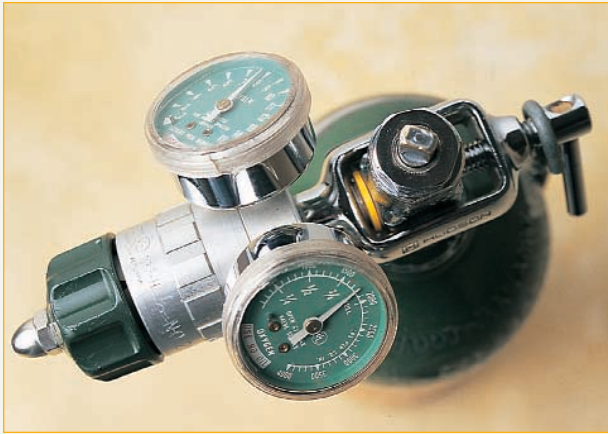
Figure 7-27 The Bourdon-gauge flowmeter is not affected by gravity and can be used in any position.
